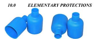
**DD0015-CV** bush covers guarantee protection against corrosion on elementary anchorages, both on temporary and on permanent anchors. DD0015-CV are particularly effective on applications with temporary anchors in several and subjected to several tensioning phases, as they protect: bush, wedge and strand against corrosion, making retensioning easier.
